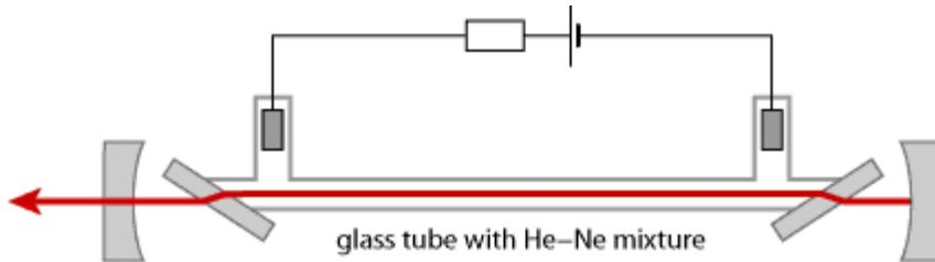
The discharge current is limited to about 5 mA by a 91 kW ballast resistor.
