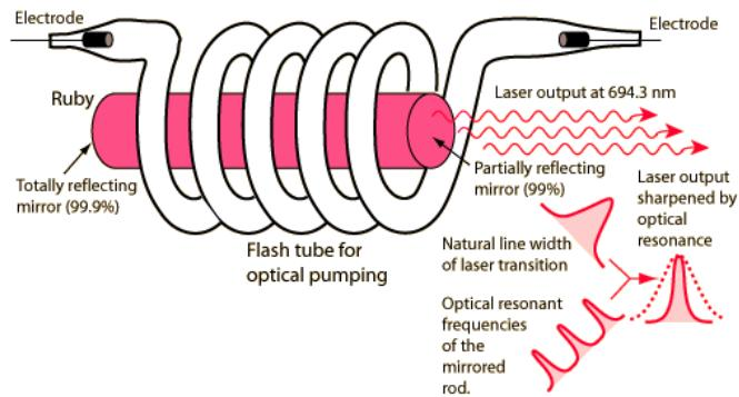
Ruby laser rod is a synthetic  $\text{Al}_2\text{O}_3$  crystal, doped with chromium ions.  $\text{Cr}^{3+}$  ions are the actual active centers and have a set of three energy levels suitable for realizing lasing action whereas aluminum and oxygen atoms are inert.
