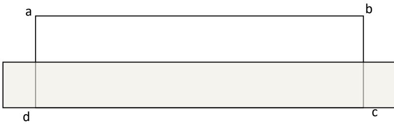
Field inside the conductor are zero.
