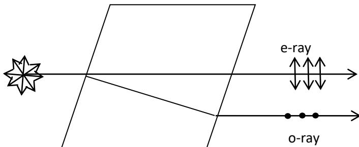
The phenomena causing two refracted rays by a crystal is called birefringence. The two rays produced are linearly polarized in mutually polarized direction. One ray obeys Snell's law and is called the ordinary ray and other ray does not obey the snell's law and is called the extraordinary ray.
